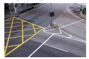
In Kent, yellow box markings have historically been overused and are expensive to install and maintain. To maintain the usefulness of yellow box markings the marking will only be considered for installation at specific locations.
